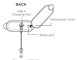
Charge via USB AC adapter (not included) or other powered USB port
