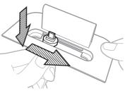
5. Plug in the micro USB cable and wrap the cord. (also a good time to insert the audio cable, described on pg. 7)
