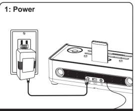
Attach AC adaptor cable to DC jack on back of the unit and plug the other end into a wall socket. Remove pull tab from the backup battery compartment on the bottom of the unit. Extend FM antenna for best reception.
