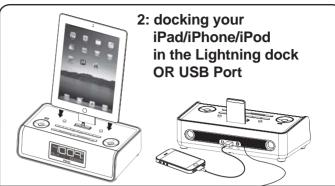
While the dock accommodates most cases, you may need to remove your case for proper docking. Gently dock any iPad, iPhone or iPod with Lightning connector onto the Lightning dock on top of the unit. The device will charge while docked. Press the >II Dock Button on the unit to play your iPad/iPhone/iPod. Connect an iPad, iPhone or iPod to the USB Port on the back of unit using the connecting cable that came with it to charge and play (press the >II USB Button).
