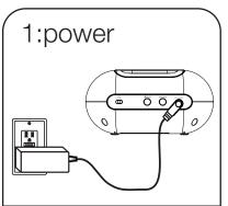
Plug the AC cable into the adapter jack in the back of the unit and the plug into a working wall socket.
