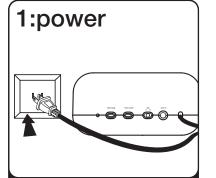
Plug the AC cord into a working wall socket.
