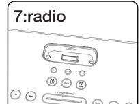
Press the Radio/Aux button as needed to select AM/FM band. Press the Forward or Reverse Button to tune in a station. See page 5 for programming presets.
