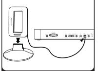
Snap the AM antenna into the provided stand, then plug the antenna cable into the socket on the back of the iH51. Move the antenna 12" away.
