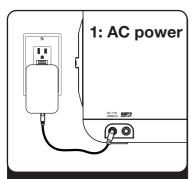
Attach AC adaptor cable to jack on back of the iH15 and plug the other end into a wall socket to play and charge iPhone/iPod
