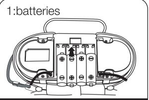
Open battery compartment and insert 4 "AA" batteries as indicated on diagram. Unit can now play iPod. Batteries will not charge iPod.
