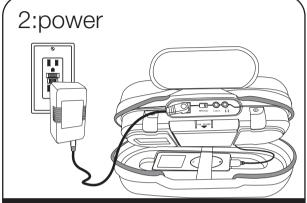
Attach AC adaptor cable to jack on top of the iH19 and plug the other end into a working wall socket to charge and play iPod. Does not charge batteries.
