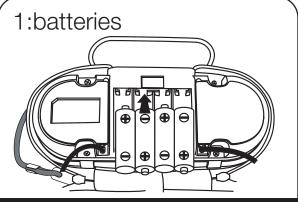
Open the battery compartment and insert 4 "AA" batteries as indicated on diagram in compartment. Unit can now play iPod. Batteries will not charge iPod.
