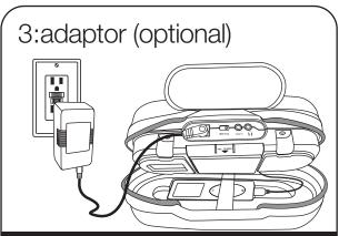
Attach optional AC adaptor (sold separately) to the DC jack on top of the iH13 and plug the other end into a working wall socket to charge and play iPod. Does not charge batteries.
