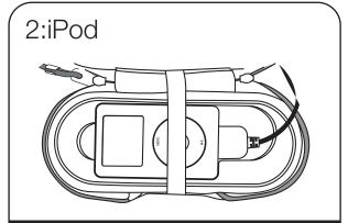
Gently insert connector plug into iPod and place iPod in iH13 docking pocket. To release iPod, press both sides of connector plug.
