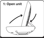
**To open** the iP49, grasp the front lid of the unit and gently pull upwards and release into lid rest.
