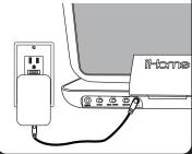
Attach AC adaptor cable to the DC jack on back of the iP49 and plug the other end into a working wall socket to play and charge iPhone/iPod and to charge the internal battery.
