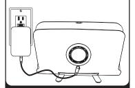
Attach optional AC adaptor cable to jack on back of the iHM8 and plug the other end into a wall socket to play.
