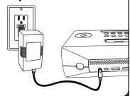
Attach AC adaptor cable to DC jack on back of the iP87 and plug the other end into a wall socket.
