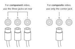
iPod classic, 3G iPod nano, 4G iPod nano, 2G iPod touch, iPhone 3GS: These iPod models can output progressive scan component video.
