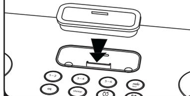
Select the dock insert for your iPhone or iPod® model from the table below and place insert in dock. **Never dock an iPhone/iPod without an insert in place.**
