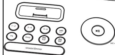
Press the Radio button and press again to select AM/FM band. Turn the Set Wheel to tune in a station. See page 4 for programming presets.
