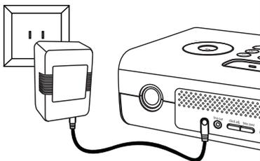
Attach AC adaptor cable to DC jack on back of the iP97 and plug the other end into a wall socket.
