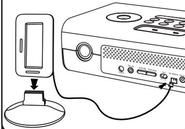
Snap AM antenna into provided stand, then plug antenna cable into socket on back of iP97. Move antenna 12" away.
