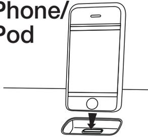
Insert an iPhone or iPod into the dock with proper insert (iPhone/iPod must not be in a skin or case). The iPhone/iPod will charge while docked. Press the ►|| Button on the iP97 to play your iPhone/iPod.
