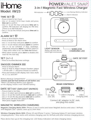
Rapid blinking LED: Device is not charging (reposition device) Slow blinking LED: Device is charging
