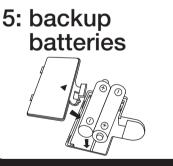
Remove the battery compartment door on the bottom of the receiver and insert 2 AA batteries (match + and - polarity to diagram in compartment). Replace door.
