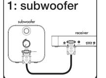
Connect the provided connector cable from the back of the subwoofer to the back of the receiver and tighten screws.
