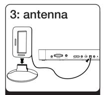
Snap the AM antenna into the provided stand, then plug the antenna cable into the socket on the back of the iP51. Move the antenna 12" away.
