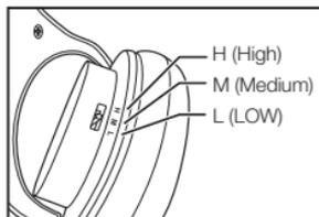
The volume switch is located on the inside of the left ear cup. Before use, have an adult use the tip of a pencil, paper clip, or other small tool to slide the switch to set the headphone volume to High, Medium or Low.
