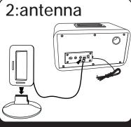
Snap AM antenna into provided stand, then plug antenna cable into socket on back of unit. Move antenna 12" away.
